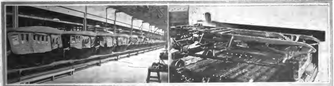
Left—View in Maxwell factory. Each body is a step nearer completion. They are moving gradually to the point where they will be picked up by an electric hoist and set on their chassis, as the latter reach that point in their growth into complete automobiles. Right—Painted chassis just entering the drying oven. In 30 min. the moving chain will pull it out dry at the other end, and the work of assembly will continue again. Another follows it only a few feet away
